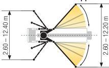
Dimensions can differ depending on configuration. Support width based on center of support leg. Diameter of swivel plate 350 mm.
